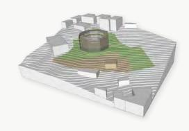
The initial concept was of a central courtyard connected to outer gardens. This proved difficult due to the topography and outline of the site. The concept evolved, with the first floor becoming an extension of the green areas outside. It serves as a link them to the inner garden, and each floor retreats, creating balconies with gardens and allowing plenty of light.
